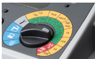
Robust rotary switches with safe and understandable colour coding
